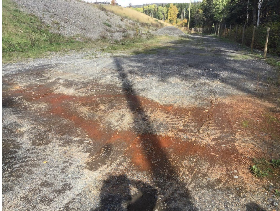
Photo 13: Kitwanga Landfill leachate breakout near MW22-03, looking north, September 27, 2022
