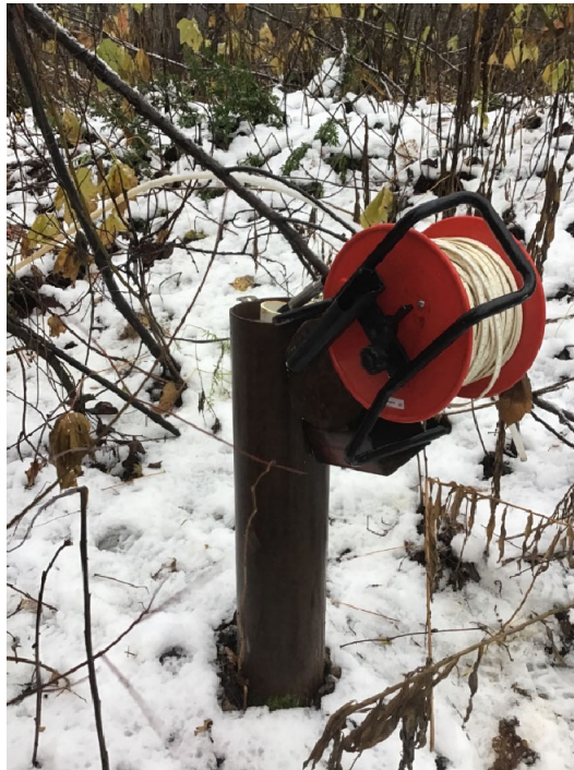
Photo 14: Meziadin Landfill MW-01AB, dual well head, October 26, 2022
