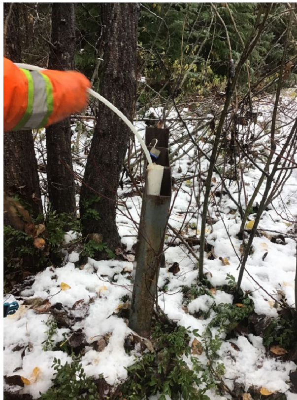
Photo 20: Meziadin Landfill MW-04, well monument, October 26, 2022
